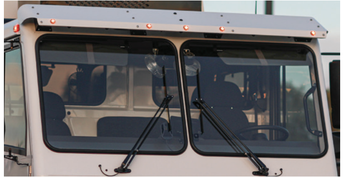
Large, flat, glass windshield; simple to replace and cost effective compared to complex, curved glass
