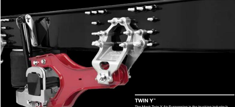
The Mack Twin Y Air Suspension is the trucking industry's first suspension to utilize an innovative Y-shaped highstrength steel design. The Twin Y is up to 400 pounds lighter than other air suspensions, offering customers a significantly lighter weight option. In addition to cutting weight and saving fuel, the Twin Y delivers unmatched comfort and handling for highway customers desiring a smoother, more stable ride.
